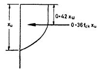
FIG. 4 STRESS BLOCK PARAMETERS
