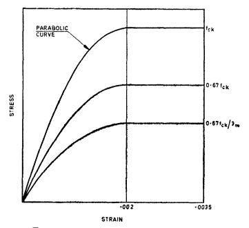
FIG. 3 STRESS STRAIN CURVE FOR CONCRETE
