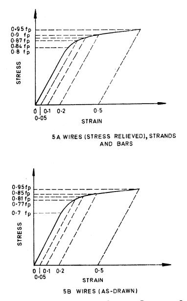
FIG. 5 REPRESENTATIVE STRESS STRAIN CURVES FOR PRESTRESSING STEELS
