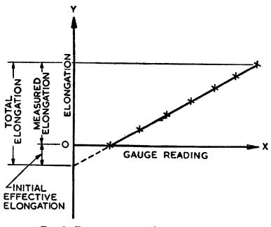
FIG. 2 DETERMINATION OF ACTUAL ELONGATION
